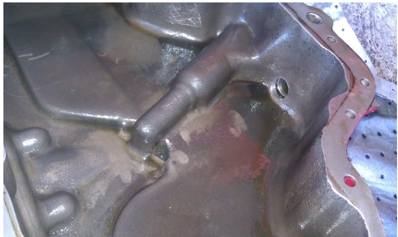
photo shows disabled oil pickup (center) and new pickup at the aft end of the pan (right)
