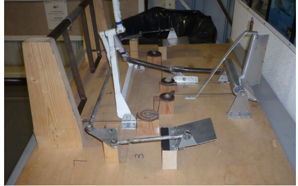
Contraption to show common flaws in Control Linkage
