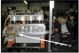
Imagine having to control the airplane and reach for a handle on the magneto with your foot to reduce the power to land. And we think we have it bad in a strong crosswind!
