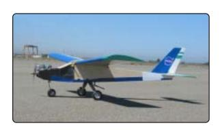
autopilot that provides state information. Software on the PC 104 is used to control of the aircraft via a two-way air to ground control link and a servo control switch. The aircraft is flown up to altitude using conventional RC control then "handed over" to the computer-based operator on the ground.
