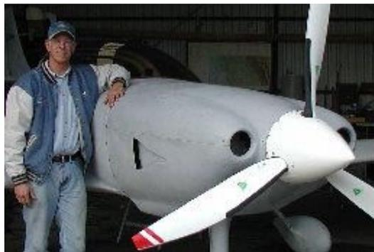
N203AW is not your standard aircraft. It flies at 203 mph. On Final Approach, Andy is at 100kts. The Legacy cruises at 170kts at 55% power and holds 65 gallons of fuel. Stall speed is 63kts. The engine is a Turbo Normalized IO-360.
