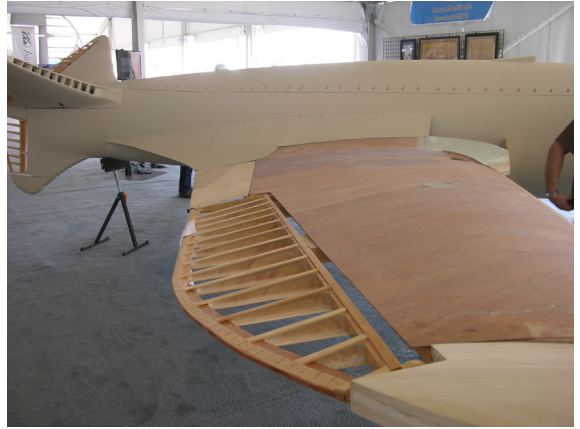
Details of the Bugatti replica wing and elevator
