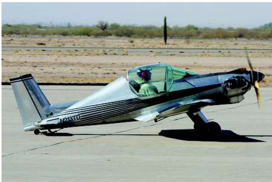
The factory H5 is a taildragger, and sported the side-opening canopy, and lower turtledeck.
