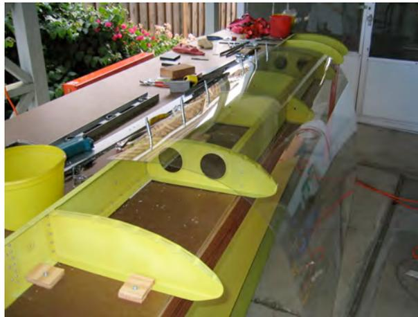
Next he laid out and drilled the holes thru the polycarb into the center of the rib flanges where required. He then removed the polycarb sheet and laid it on the metal skin that he was going to use and drilled two holes at the ends of the spar rivet row to use as the locator and clecoed the metal and the polycarb onto the wing. He then ,using the polycarb as a location tool, drilled each hole where there was a hole
