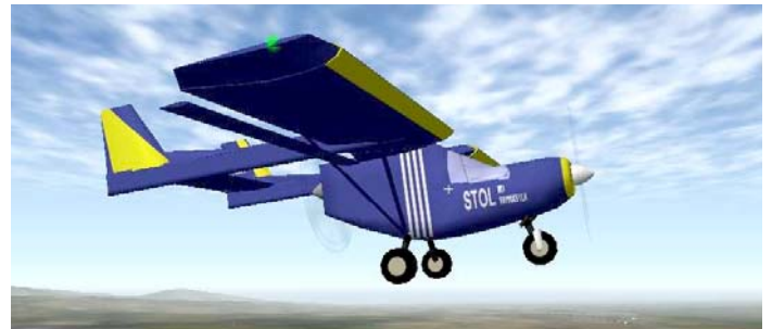
ZenMaster - Rear Engine is mounted higher than the front for steep climb rotation.
